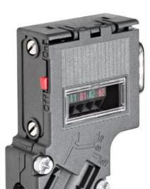
PROFIBUS bus connector, RS485, screw, without PG socket, 35° PROFIBUS bus connector, RS485, screw, without PG socket, 35° SIMATIC DP,BUS CONNECTOR FOR PROFIBUS UP TO 12 MBIT/S WITH TILTED CABLE OUTLET, 15,8 X 54 X 39,5 MM (WXHXD), TERMINAT. RESIST. WITH ISOLAT. FUNCTION, WITHOUT PG SOCKET
